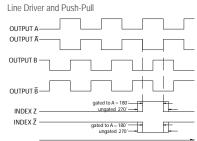
CLOCKWISE ROTATION AS VIEWED FROM THE MOUNTING FACE NOTE: ALL DEGREE REFERENCES ARE ELECTRICAL DEGREES. ALL DEGREE REPERENCES ARE ELECTRICAL DEGREES. WAVEFORM SHOWN WITH OPTIONAL COMPLEMENTARY SIGNALS  $\overline{A}, \overline{B}, \overline{Z}$  FOR HV OUTPUT ONLY.
