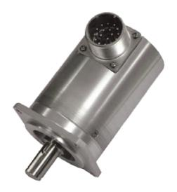
Model DR86A is an extra heavy duty unit that employs a highly reliable Opto-ASIC encoder module mounted within a rugged mechanical housing. The heavy duty sealed bearings, together with double O-ring sealing, makes this encoder a serious and reliable alternative to a wide range of machine tool encoders, and at an economical price.
